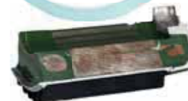
Insulated motor winding cross section
